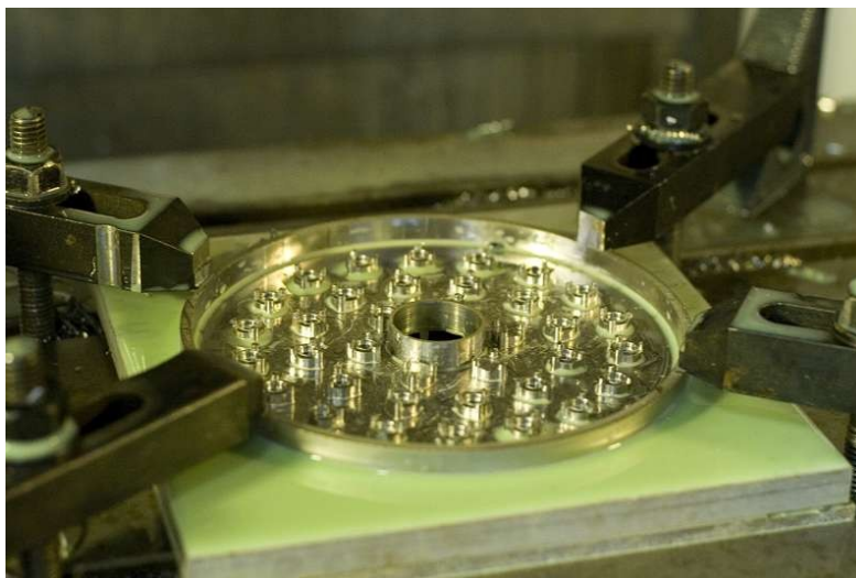
An engine injector plate being milled.
